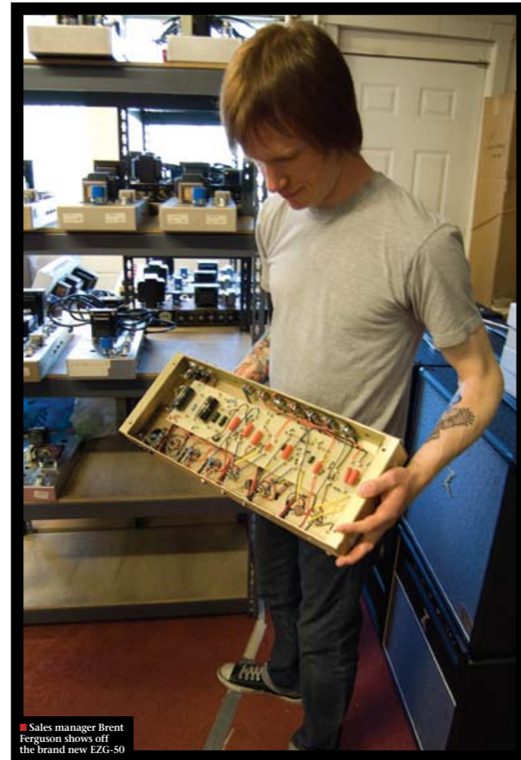
■ The amps are all wired by hand the old-fashioned way
