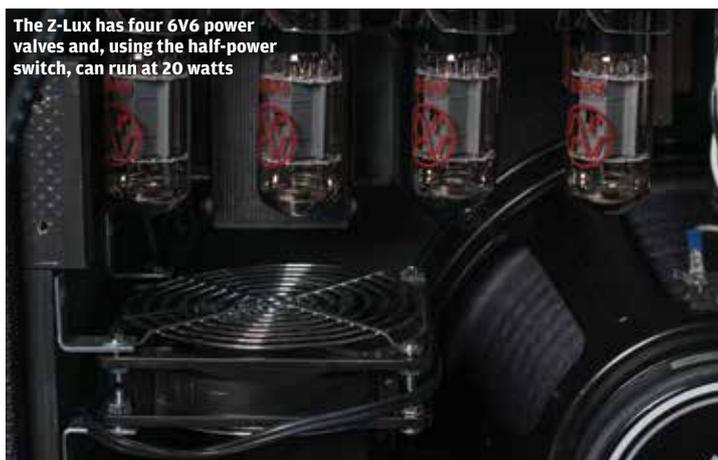
The Z-Lux has four 6V6 power valves and, using the half-power switch, can run at 20 watts
