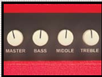
■ Unlike the other two amps, the MAZ 18 Jr NR features a master volume control
