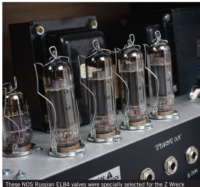
These NOS Russian EL84 valves were specially selected for the Z Wreck
