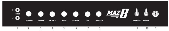
1.) INPUT: Plug guitar in here. HI is for normal use. LO has 3dB less gain. Use LO with humbuker equipped guitars for a cleaner sound.
