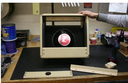
6. Use an Exacto knife to cut out the 4 chassis mounting holes on top of the cab. These holes are already drilled.
