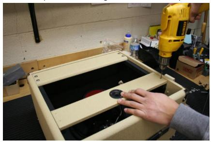
8. Mount chassis using the 4 screws from your old head or combo.
