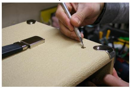
7. Lay cabinet flat and position upper back panel even with the side mounting rails. Drill out 4 pilot holes using 1/8" drill bit. Set panel aside.
