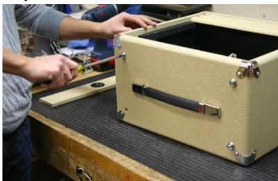
9. Attach upper back panel and 1/4" jack. You may choose to use a short speaker cable to connect the jack and chassis. You may also install a new speaker lead with a 1/4" plug to go directly from the speaker to the chassis.
